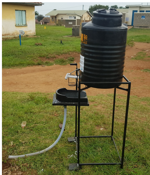
Figure 5.7: Foot operated Hand Washing Facility
